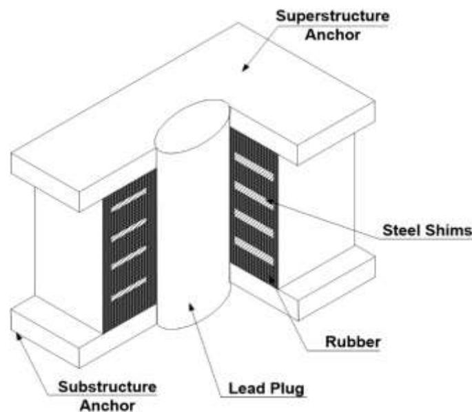
*Figure 4: Lead – plug isolators.*
