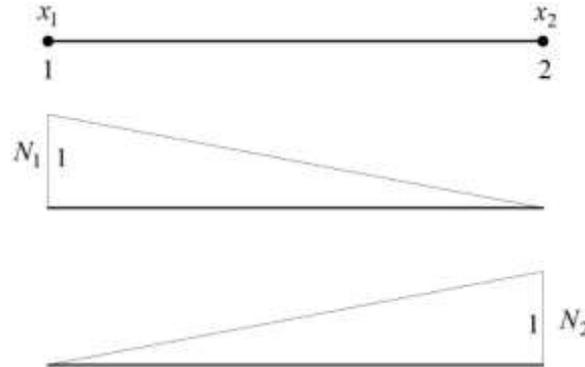
Figure 11: Beam element shape functions.
