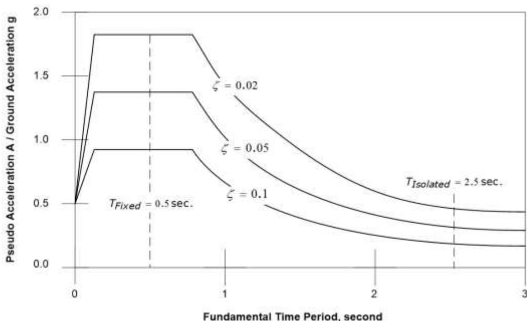
Figure 1: Design spectrum and spectral ordinates for fixed – base and base - isolated systems (2).
