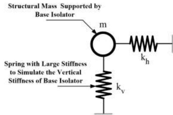
Figure 6: Two-spring model of base isolator.
