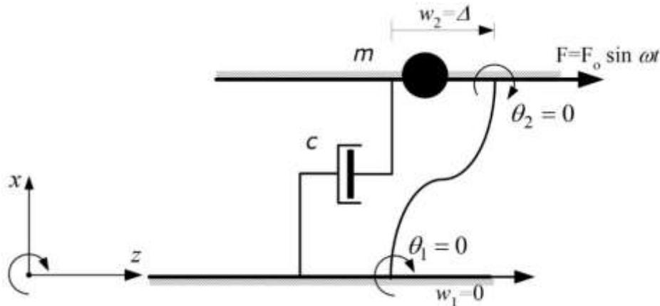
Figurer 12: Deep frame element with viscous damping.
