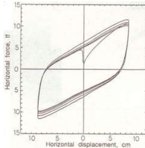
Figure 5: Typical Force – Displacement Relation of Lead - Plug Rubber Bearing (4).
