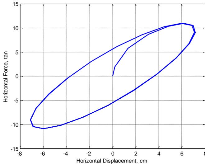
Figure 9: Response of lead-plug rubber bearing based on equivalent viscous damping model.
