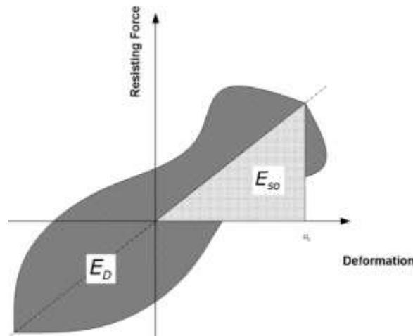
**Figure 7: Energy dissipation in a cycle of harmonic vibration determined from experiment on base isolator.**
