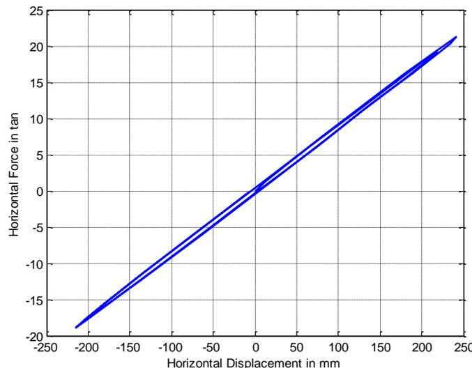
**Figure 8: Response of low damping rubber bearing based on equivalent viscous damping model.**
